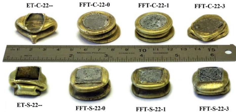
Fig. 9. Behavior of progressive plastic buckling foam-filled brass tubes with circle and square cross-section after uniaxial compressive loading.
