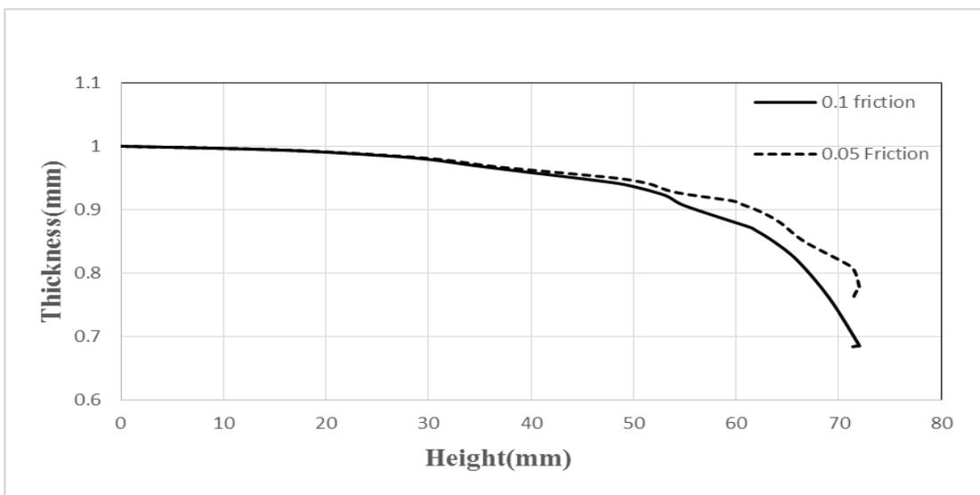
Fig. 3. The effect of friction on the bottom sheet thickness variation.
