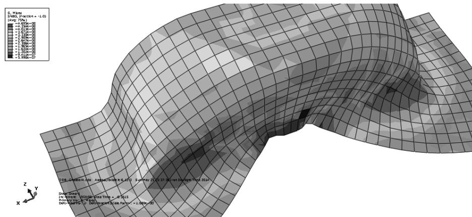
Fig. 8. Schematic of wrinkles caused due to the shortness of the mold.
