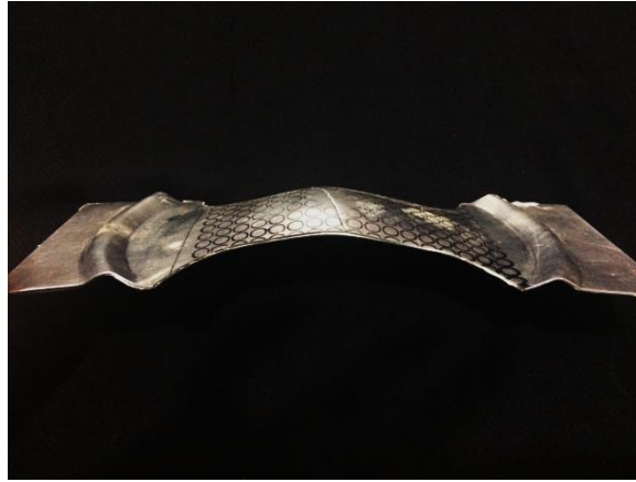
Fig. 4. The 75 mm×200 mm specimen after forming.
