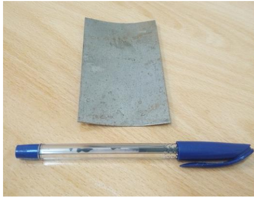
Fig. 1. A specimen after rolling and heat treatment with radius of curvature of 120 mm.
