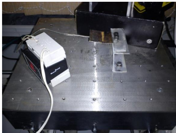
Fig. 6. Experimental setup for measuring temperature profiles on the bottom surface under the heat line and on the top surface with 1 mm distance from the center of heat line with thermocouple.
