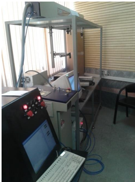
Fig. 2. Experimental setup for laser forming of a dome and saddle shapes.
