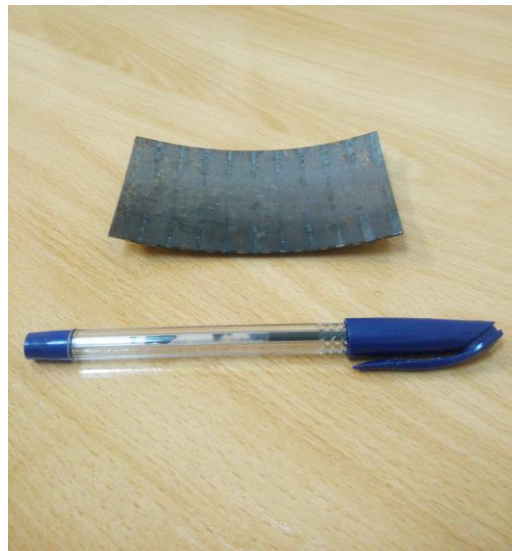
Fig. 4. Obtained dome shaped part with the proposed irradiating scheme.
