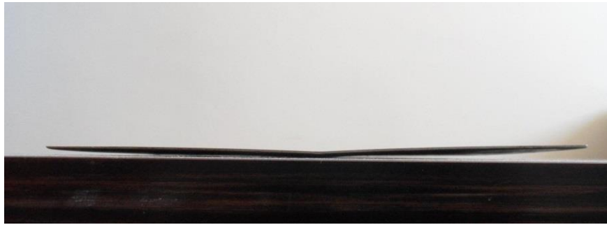
Fig. 2. The tailor machined blank after laser forming.
