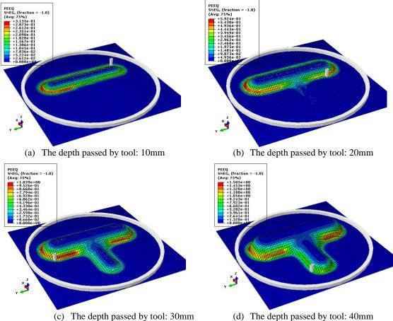
Fig. 10 Plastic strain counters induced in sheet during TPIF of the saddle-like part.
