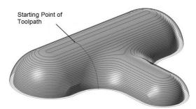
Fig. 3. Tool-path obtained from CAM software on punch designed for part.
