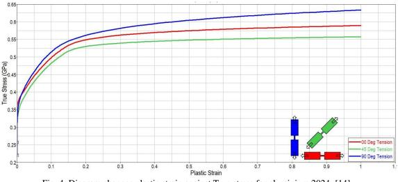
Fig. 4. Diagram changes plastic strain against True stress for aluminium 2024 [14].
