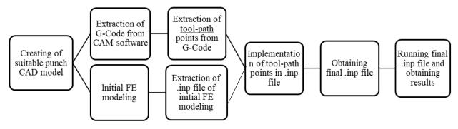
Fig. 2. General workflow of FE modeling and used software.
