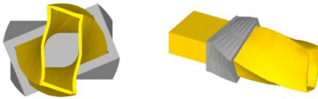
Fig. 8. The amount of twist for the 50 mm WR90 waveguide by means of a 12.5 mm and 22.5° twist die, with an ultimate angle of twist of 83°.
