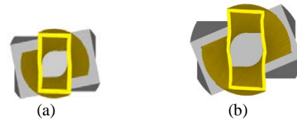
Fig. 13. The amount of observed distortion in 100 mm length and cross section of: (a) 12.95 mm × 6.477 mm (WR51), (b) 22.86 mm × 10.16 mm (WR90).
