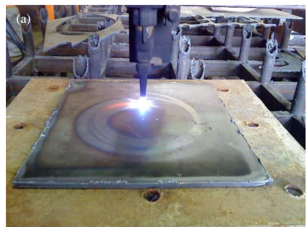
Fig. 1. a) The heat irradiation set-up b) sample of flame formed saddle-shaped surfaces with the spiral irradiating scheme c) schematic illustration of the spiral path movement.
