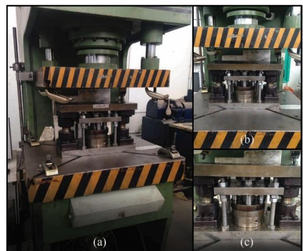
Fig. 7. The experimental equipment, (a) 60 tons hydraulic press machine, (b) deep-drawing die that installed on the press machine, (c) die.
