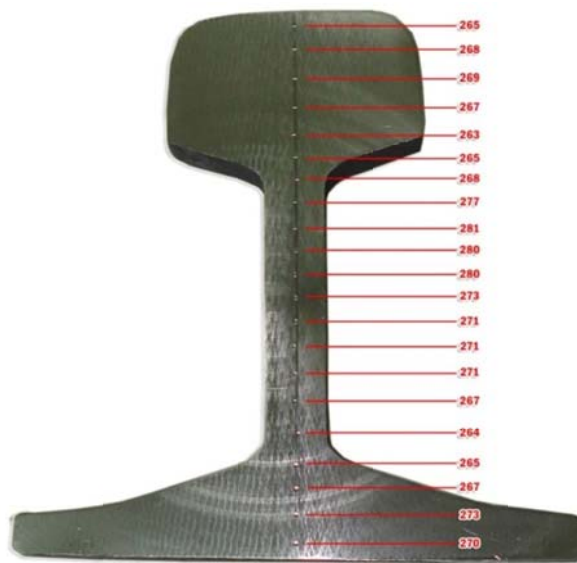
Fig. 9. Result of hardness test, (numbers in HB)
