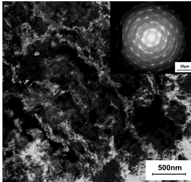
Fig. 3. TEM micrograph showing the limited twin density in 70/30 brass after three ARB cycles.
