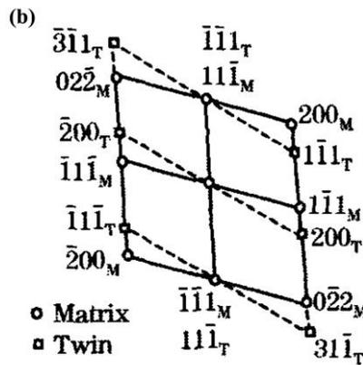
Fig. 1. a) TEM micrograph of the dislocations and mechanical twins in 70/30 brass after one ARB cycle (RD= Rolling Direction, TD= Transverse Direction) and b) diffraction analysis.
