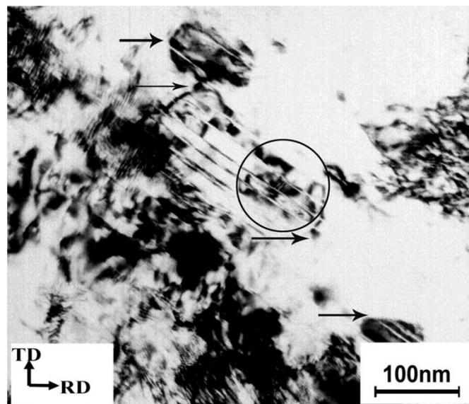
Fig. 4 TEM micrograph illustrating nanotwin formation in nano-grains, the circled region displaying nanotwins with a “stepped” morphology.
