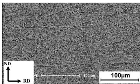
Fig. 2. Cross section SEM micrograph illustrating the shear bands in 70/30 brass after two ARB cycles.
