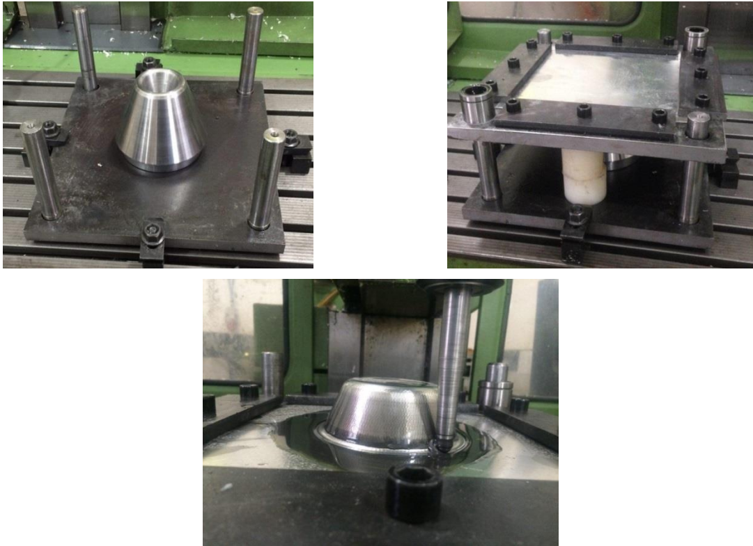
Fig. 3. The die, fixture and forming tool in the experimental work.
