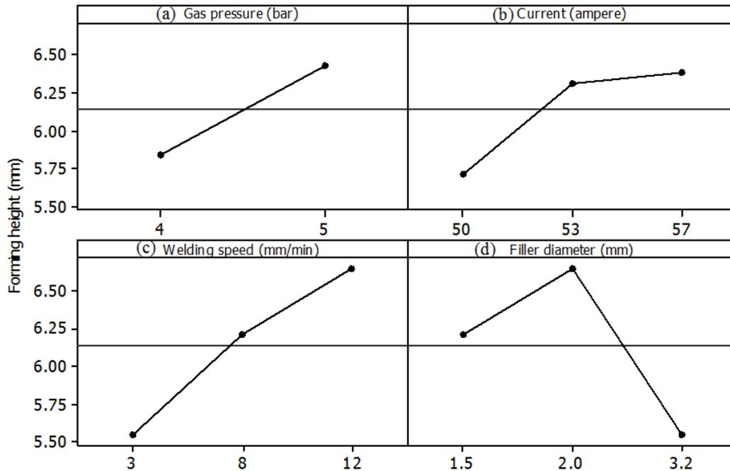
Fig. 5. Main effect plots for welding parameters via forming height of Erichsen test.
