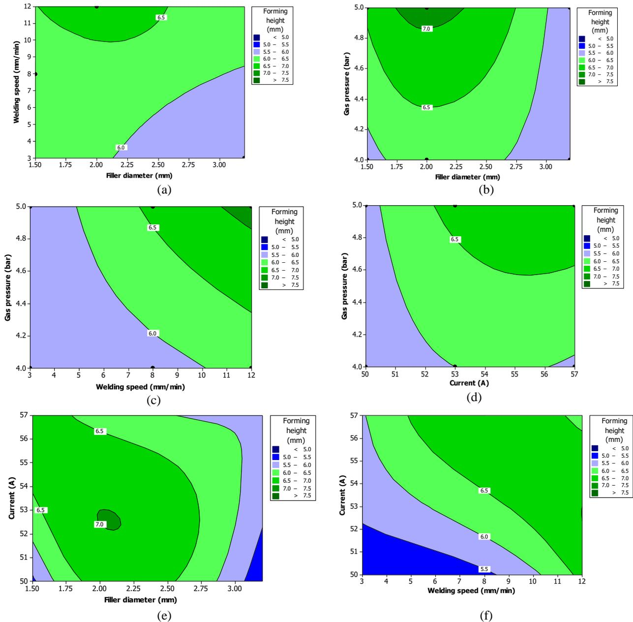
Fig. 9. Analysis of the forming height by Taguchi method.
