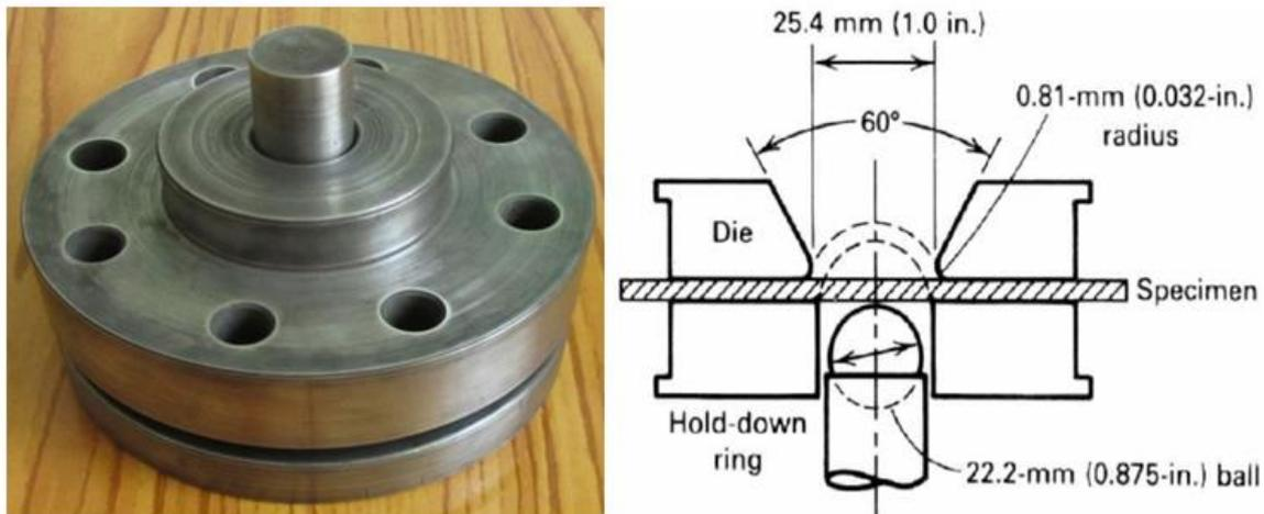
Fig. 3. Erichsen formability test setup.
