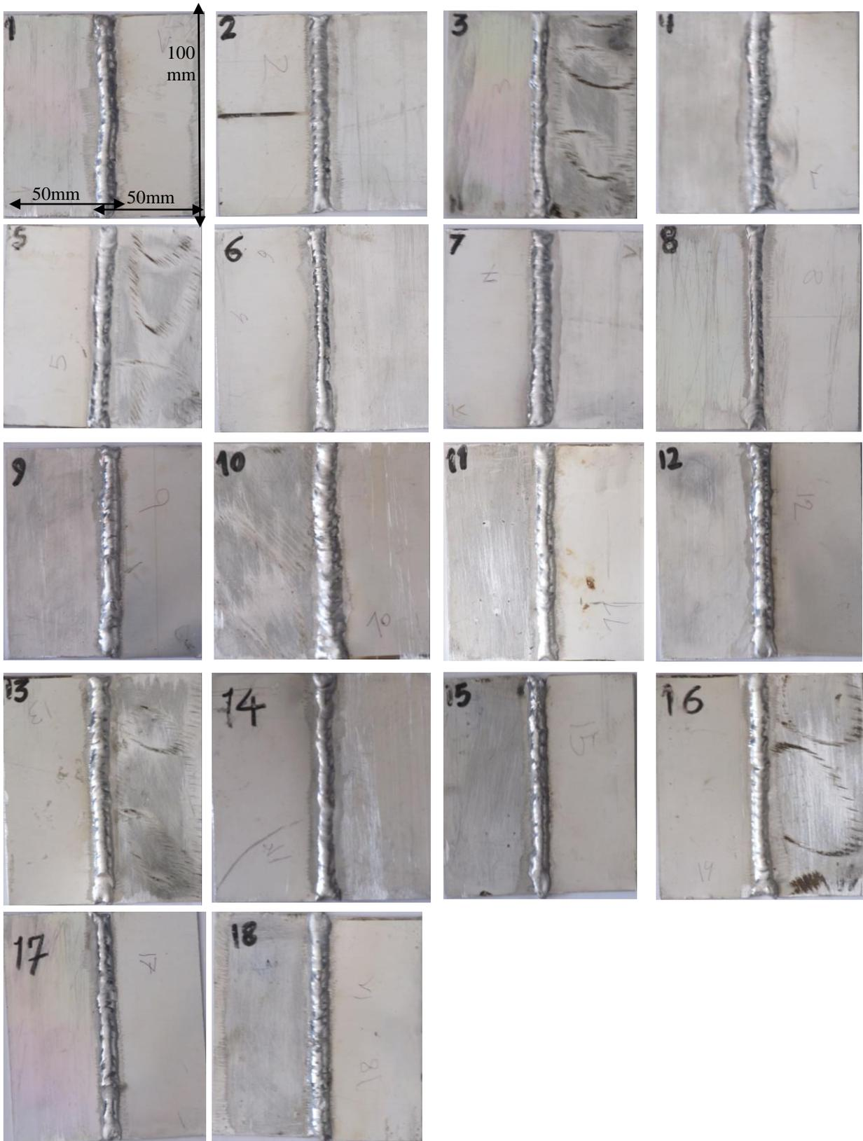
Fig. 2. TWB samples after GTAW.
