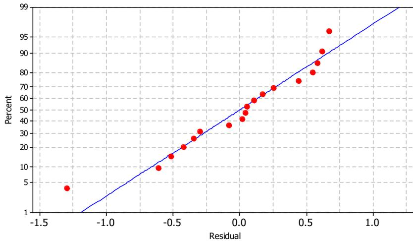
Fig. 7. Normal probability plot of residuals for forming height.
