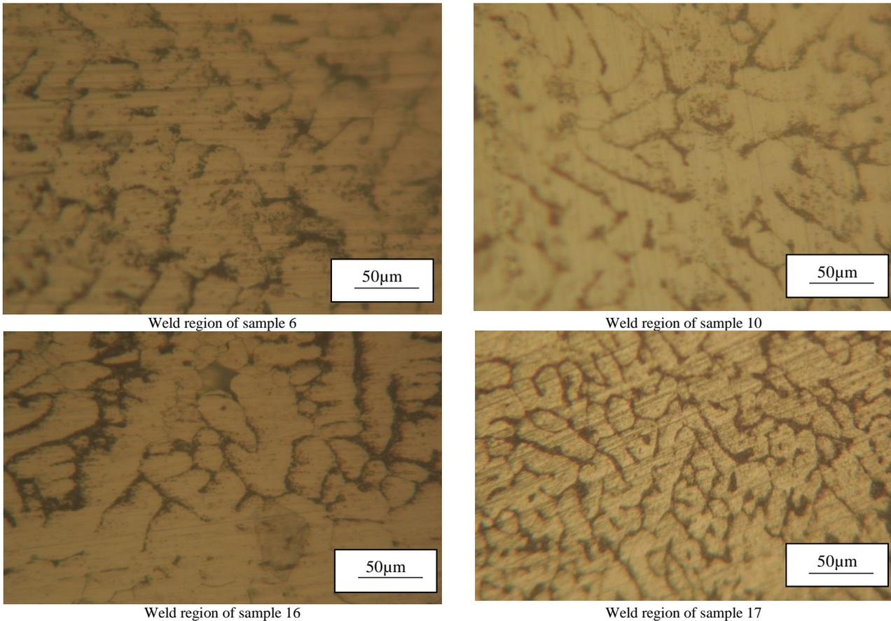
Fig. 6. Microstructure of weld region of different TWBs produced by GTAW.
