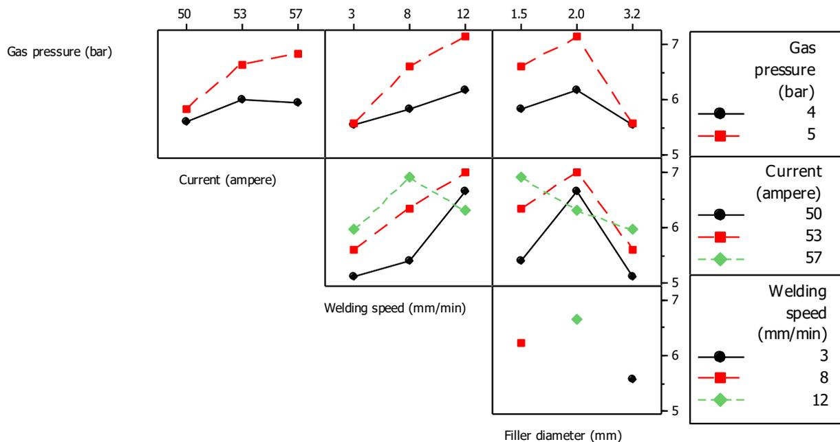
Fig. 8. Interactive effect of welding parameters on the forming height.
