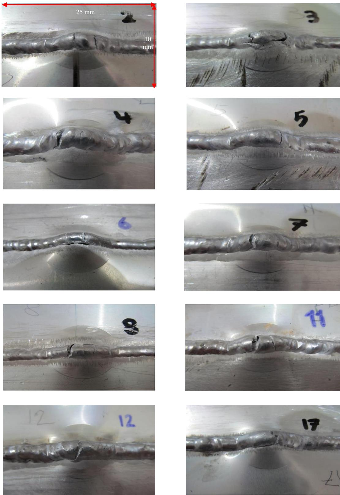
Fig. 4. TWB samples after Erichsen formability test.
