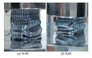
**Fig. 3.** Sequential images of the crushing process for the zinc-A356 alloy foam filled tube after (a) 10%, (b) 17%, (c) 35%, (d) 45%, (e) 58%, and (f) 65% compression.
