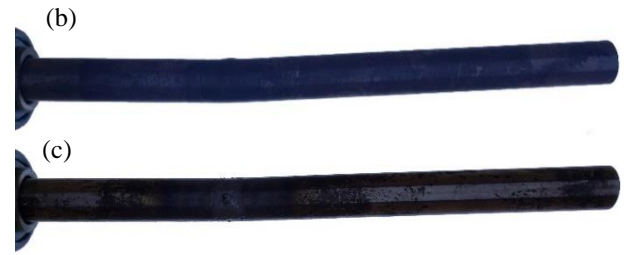
Fig. 2. (a) Comparison of the bend angle under the condition of the circumferential scanning with and without cooling after 16 passes; (b) tube after laser bending with cooling (cooling offset: 10 mm); (c) tube after bending without cooling.
