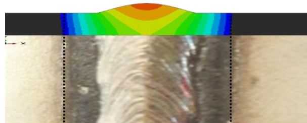
Fig. 5. Geometrical comparison of Heat Affected Zone between specimens and the FE model.
