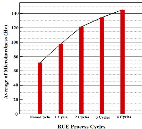
Fig. 6. The average microhardness value for the fully annealed specimen and the specimens after the RUE cycles.
