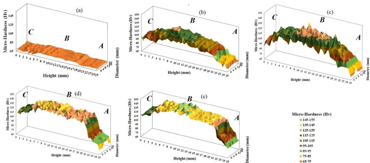
Fig. 9. Surface Micro-hardness distribution graph for fully annealed specimen and the specimens after RUE cycles.
