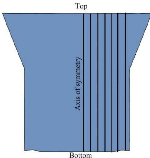
**Fig. 2.** Vertical lines with equidistant for measurement of the microhardness.
