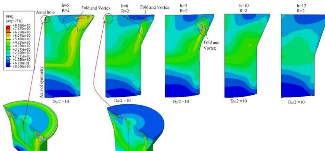
Fig. 5. The deformation pattern obtained by varying ‘h’ for an extrusion ratio (R) of 2.
