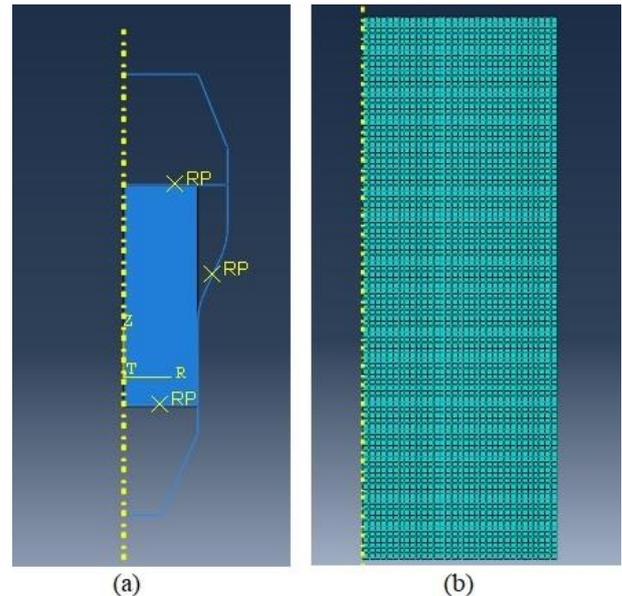
Fig. 3. (a) the assembly of RUE process simulation, (b) the meshed work-piece by Abaqus simulation.
