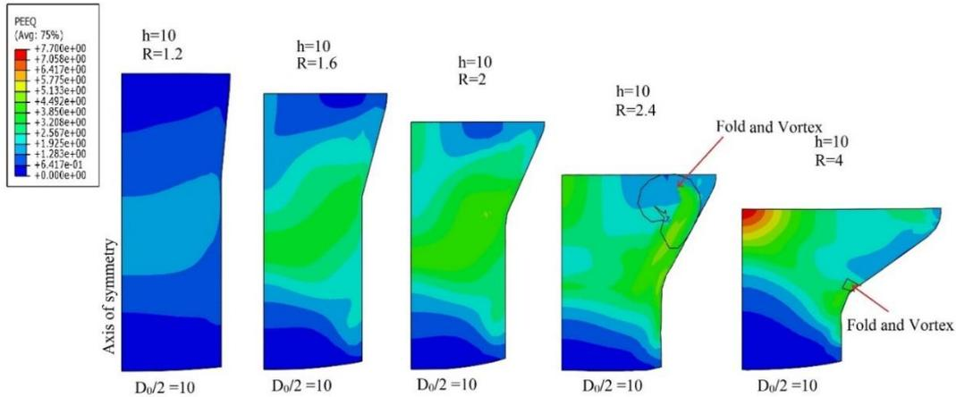
Fig. 4. The deformation pattern obtained by varying ‘R’ for a deformation zone height (h) of 10.
