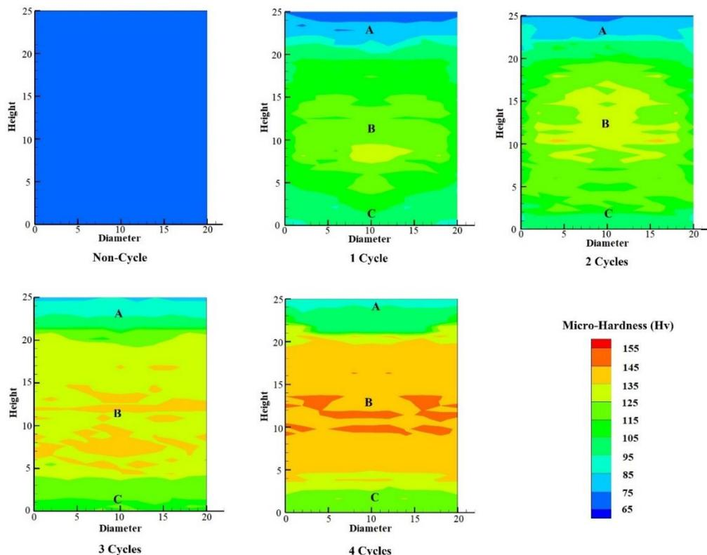
Fig. 7. Microhardness distribution for the fully annealed specimen and the specimens after the RUE cycles.
