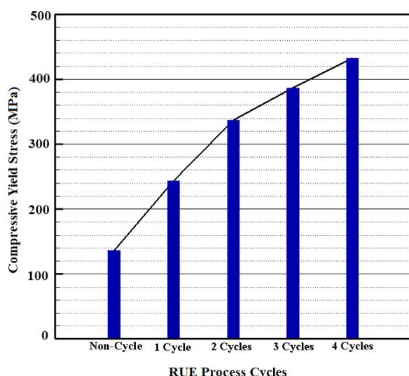
Fig. 10. Compressive yield stress of the Aluminum- magnesium 5452 alloy subjected to various cycles of the RUE process.
