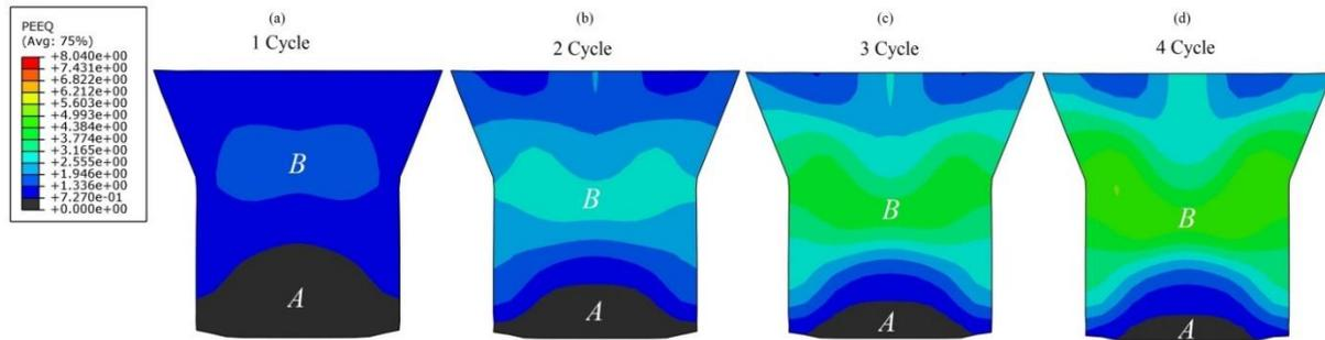
Fig. 8. The variations of the equivalent plastic strain (PEEQ in Abaqus) with an increase in the RUE cycles.
