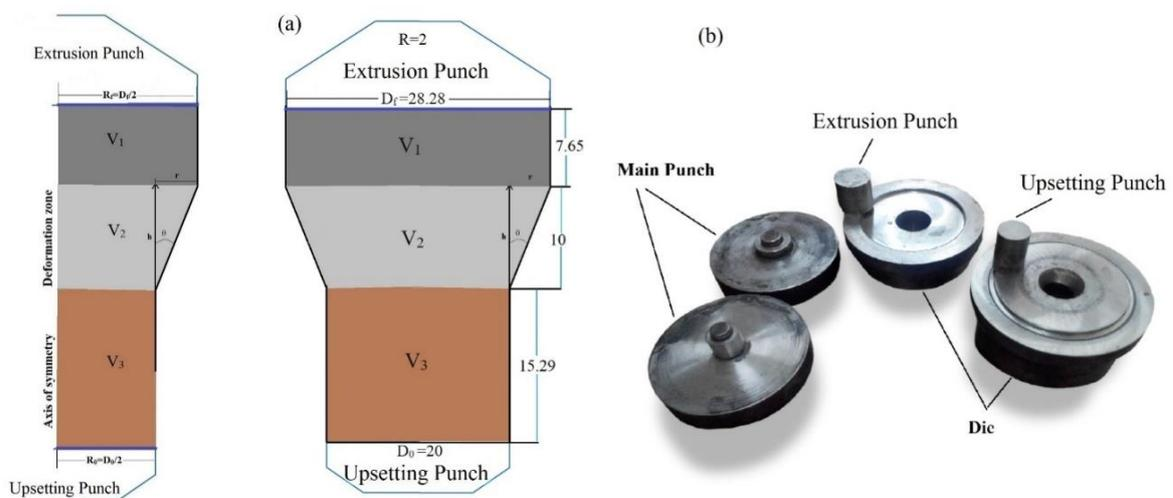
Fig. 1. Axisymmetric model of the RUE process, (a) The dimensions of the RUE die (mm) and (b) 3-D images of the RUE die.
