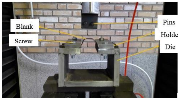
Fig. 2. The set of die and sheet on a hydraulic press ( R_d=10 mm, R_p=6 mm, D=30 and h=20 mm).
