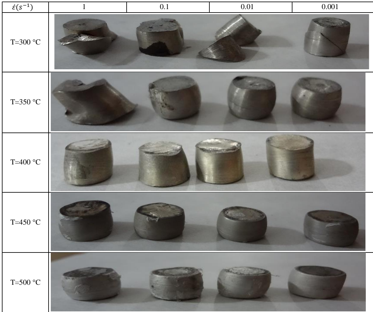
Fig. 4. Samples hot compressed at different temperatures and strain rates.
