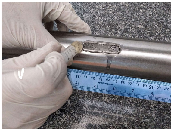
Fig. 2. Inserting a molded resin into the specimen defect, using the similar liquid resin as the adhesive.
