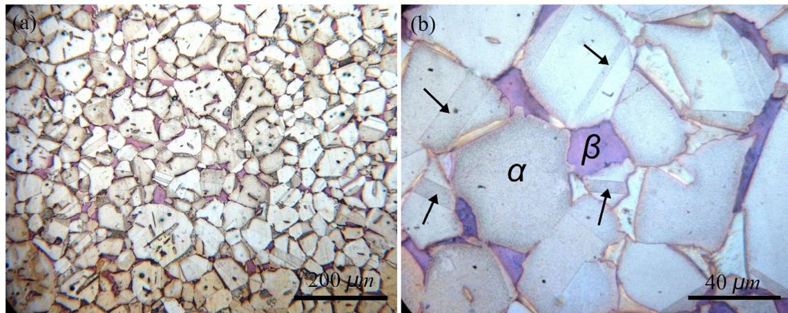
**Fig. 1.** OM images of the BM after non-equilibrium heat treatment at different magnifications: (a) low magnification and (b) high magnification. The arrows refer to the annealing twin in  $\alpha$  grains.
