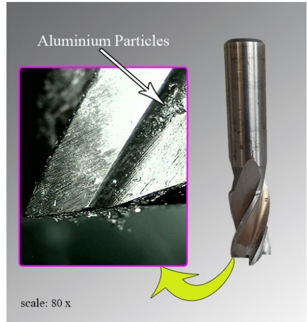
Fig. 10. Presence of piled up aluminum particles on the tool face.
