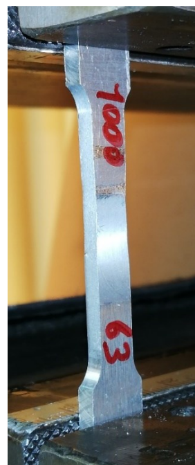
Fig. 5. Prepared tensile test FSW specimen according to ASTM E8 to determine tensile strength.
