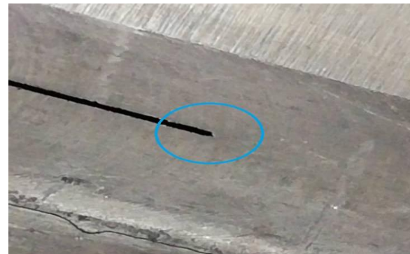
Fig. 7. The created notch using wire cut and a narrow cutter.
