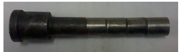
Fig. 6. The manufactured punch, divided into smaller parts.
