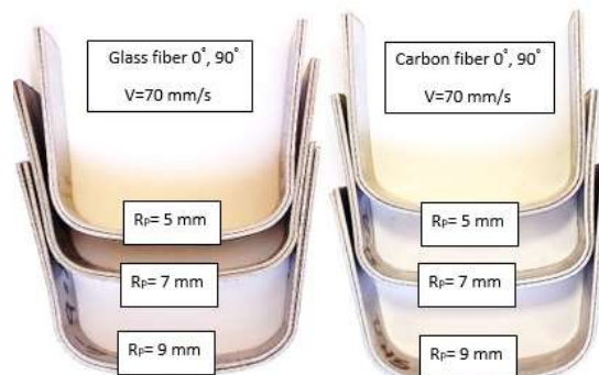
Fig. 11. Springback of experimental samples with fiber angle 0°, 90° and V=70 mm/s.
