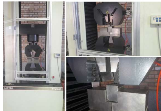
Fig. 7. Bending process using the Santam STM-600 Machine.
