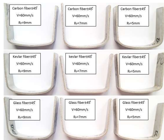
Fig. 10. Springback of experimental samples with fiber angle ±45° and V=60 mm/s.
