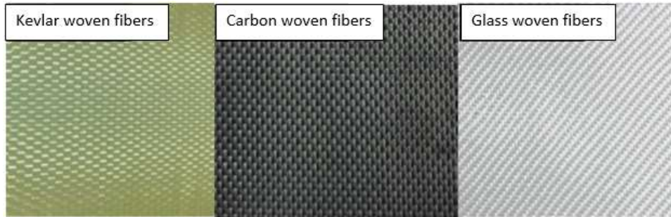
Fig. 1. Types of woven fibers used in the fabrication of FMLCs.
