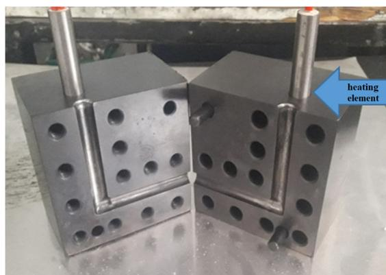
**Fig. 1.** The ECAP die set used in the present work.
