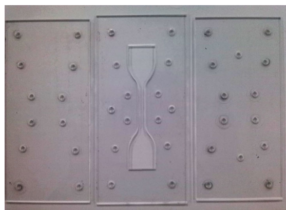
Fig. 2. PMMA mold for producing tensile standard samples.
