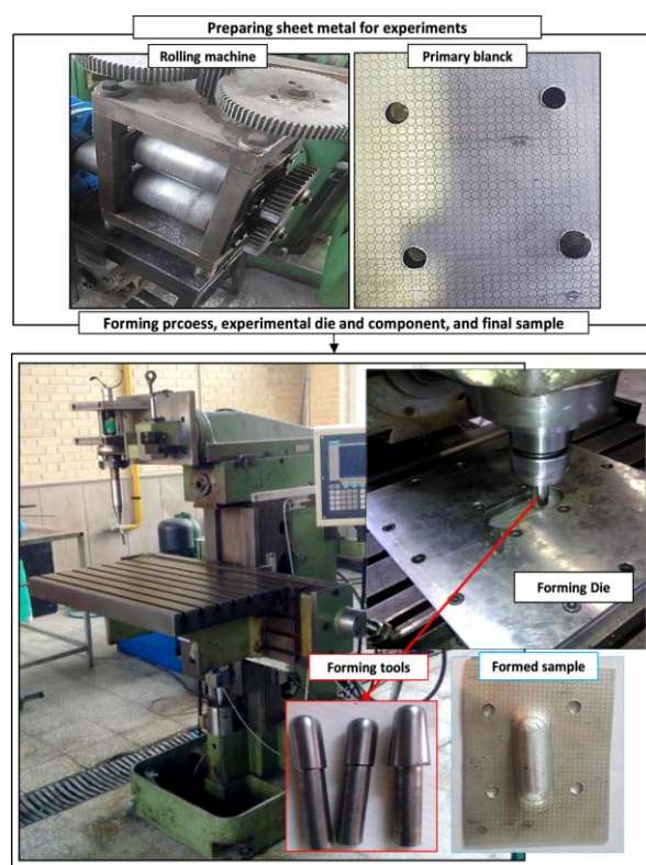
Fig. 3. Experimental equipment for the incremental forming process; initial sheet dimensions: 700 × 1000 mm.
