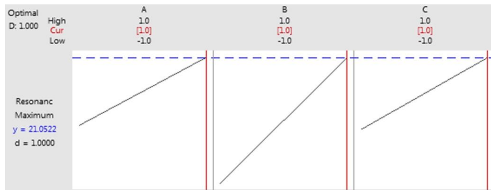
Fig. 8. Optimization results targeting the maximum resonant frequency.
