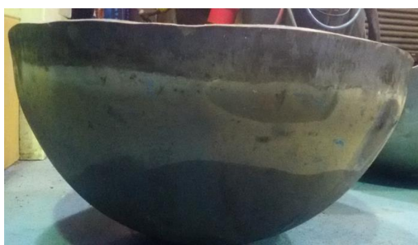
Fig. 9. Final shape of the hemisphere obtained from the hot deep drawing of CP titanium.
