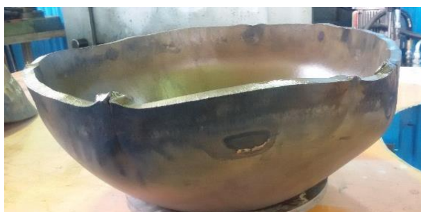
Fig. 8. Wrinkling in the blank at a temperature of 400°C and blank diameter of 600 mm.
