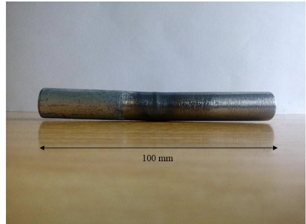
Fig. 1. A bent tube with a continuous CO 2 laser in the experiments.
