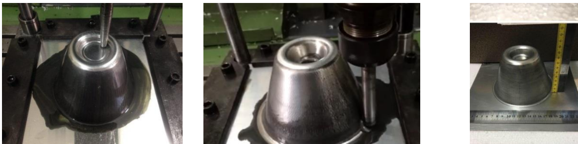
Fig. 4. Different stages of negative and positive TPIF of aluminum 3105 and the final manufactured specimen.
